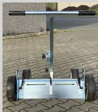
Length arm and working width adjustable by screw clamps
